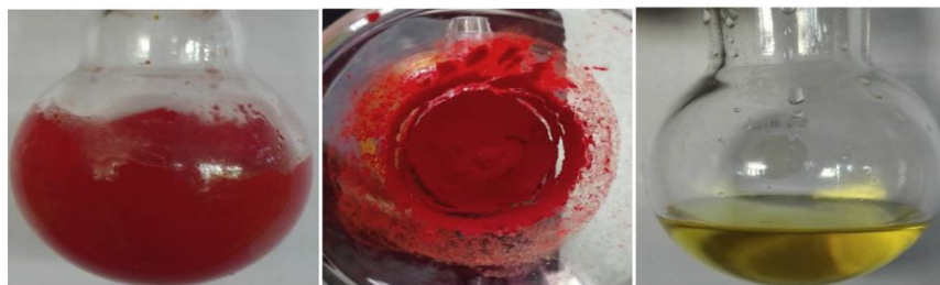
(d) Reaction mixture (after reaction); (e) The product isolated by direct filtration; (f) The recovered IL9 in aqueous.
